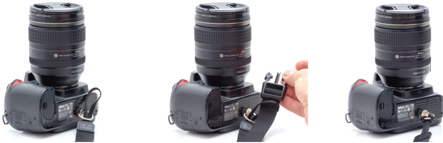
FIGURE 1: Create a girth hitch by passing the tether loop through the camera clip (left), passing the buckle through the loop (center) and finally pulling the buckle tight to secure the hitch.
