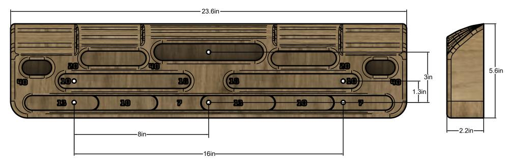
The BuddyBoard+ mounts directly to 16" spaced studs, as is typical in home construction. If direct mounting to studs, the center screws are recommended, but not required, for structural support. The screws are sized to be drilled into your studs through standard ½" drywall, or can be direct-mounted to unfinished studs. Please use only the included screws, as our engineers have certified them to carry the expected shear and pull-out loads associated with hangboard use.
